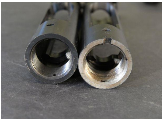
A front view of both receivers. The Savage (right) had a notch located to the bottom front edge of the receiver, this allows for indexing of lugs with an indexing pin.
