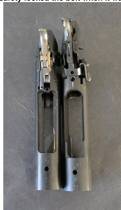
A bottom view of both receivers. Note the location of location of the action screws for both models. The Remington (left) has an action screw located at the front of the receiver and on the rear of the tang. The Savage has both screws located in front of the trigger guard. The proximity of the screws to each other on the Savage, make bedding with bottom metal a little more difficult. The magazine well on the Savage is longer.
