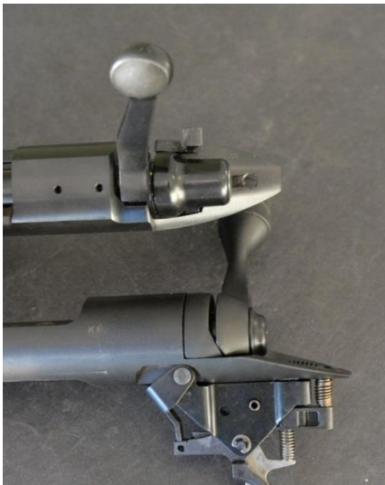
Primary extraction for the Remington 700 (top) occurs when the bolt cams against the rear of the receiver. Primary extraction for the Savage occurs when the bolt handle cams against rear baffle assembly.
