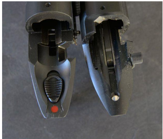
The Savage (left) uses a tang mounted three position safety. In its rear most position, the bolt is locked and rifle won't fire (Full Safe), in the middle position the bolt can be manipulated without firing the rifle (Mid Safe), when the safety is off, the bolt can be manipulated and rifle fired (Off). The bolt release lever is located on the right side of the receiver, forward of the bolt handle. The Remington 700 (right), uses a two position safety. When the lever is to the rear, the rifle cannot fire and the bolt can be manipulated, when the lever is forward, the rifle can fire and the bolt can be manipulated. Note: on older Model 700s, the safety locked the bolt when it was engaged.
