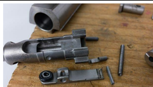
After cleaning the bolt and chamber, remove the extractor and ejector before testing headspace.
