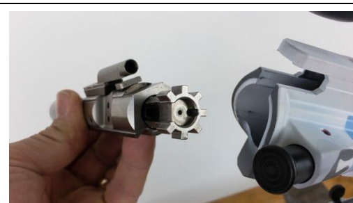
Always remove the ejector and extractor before checking headspace.
